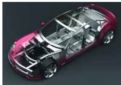
Fisker Karma electric powered vehicle is assembled using self-piercing technology
