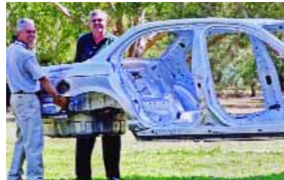
The Jaguar body is assembled using self-pierce riveting and is light enough to lift
